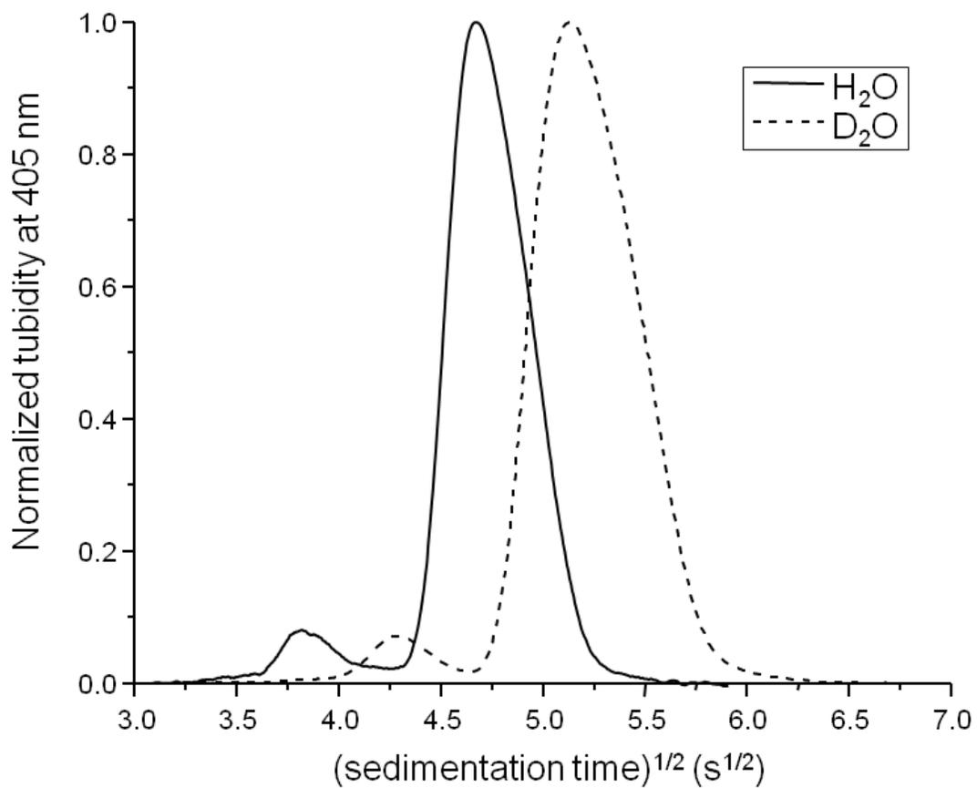
**Figure 1.** Normalized centrifugal sedimentation data for sample A in H<sub>2</sub>O-sucrose gradient (solid line) and in D<sub>2</sub>O-sucrose gradient (dashed line). Turbidity at 405 nm was normalized to the peak turbidity of the respective data set. Disc speed for both data sets was 10,000 rpm.
