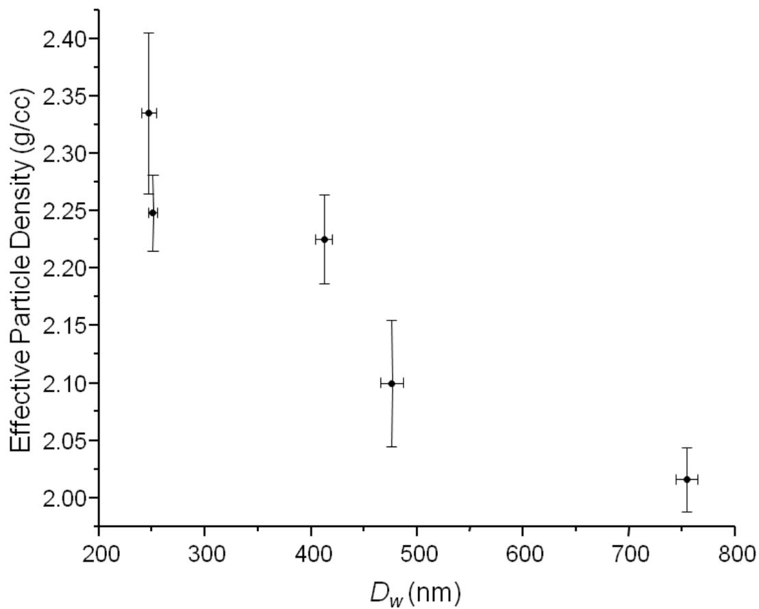
**Figure 4.** Dependence of the measured effective particle density on the weight-mean diameter,  $D_w$ . Error bars shown are  $\pm 1\sigma$  limits about the mean values represented by the solid circles.
