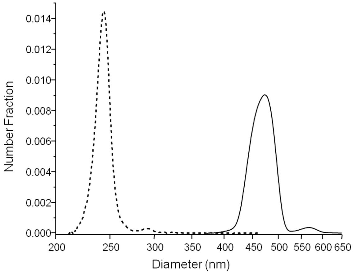
**Figure 3.** Overlay of number-mean particle size distributions for sample A (solid line) and sample B (dashed line) analyzed in a D<sub>2</sub>O-sucrose gradient and calculated with measured effective particle densities of 2.34 and 2.10 g/cc, respectively. Disc speed used for both analyses was 7,500 rpm.
