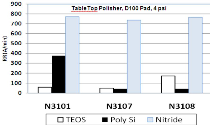
Figure 6. Comparison of silicon nitride, silicon dioxide and polysilicon removal in the N310X polishing series (2% abrasive)
