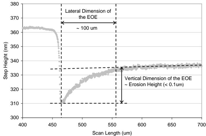
Figure 12. EOE in typical tungsten polishing
