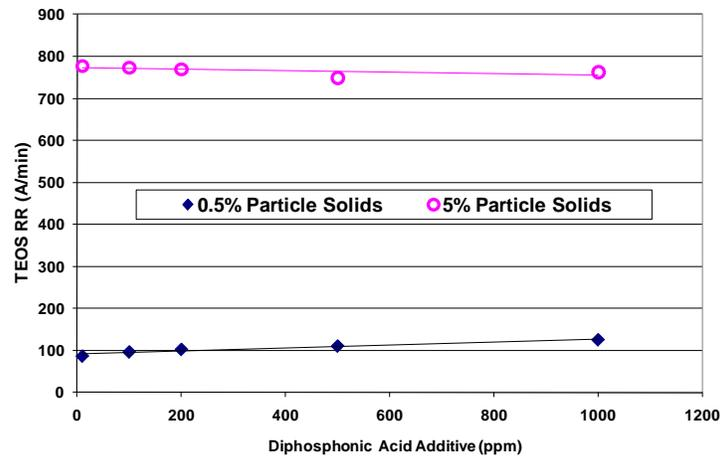
Figure 4. TEOS RR vs N1113 slurry additive level
