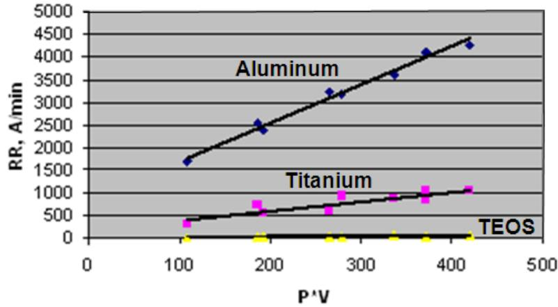
Figure 8. Polishing of aluminum in representative A71XX slurry
