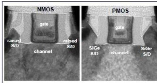
Figure 10. Intel's 32 nm NMOS and PMOS transistor structures
