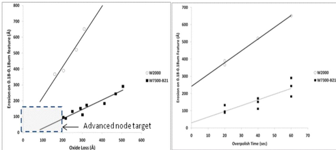
Figure 11. Topography vs Loss and Time for SS-W2000 and WIN<sup>™</sup> W7300-B21
