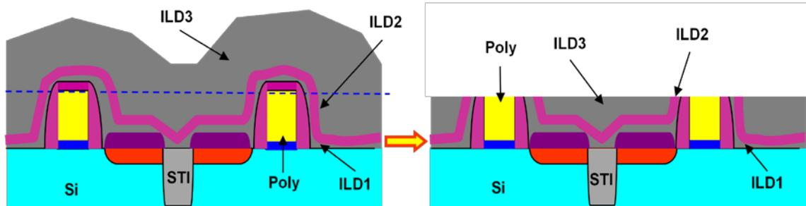
Figure 2. First CMP step clearing bulk oxide and stop on nitride. Second step nitride/oxide polish stopping on poly.
