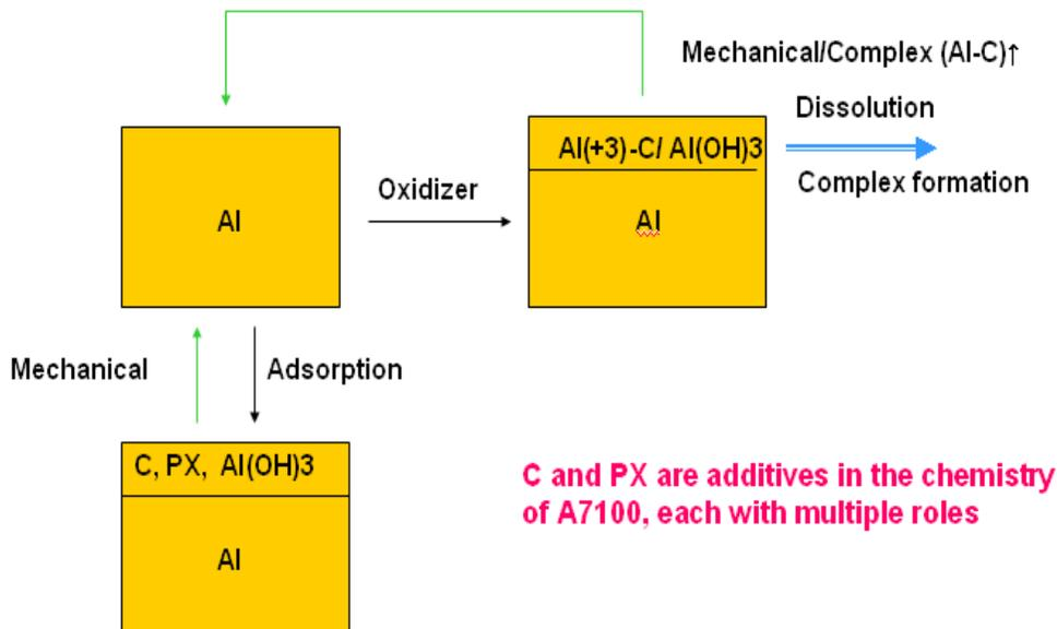
Figure 7. Simplified mechanism of polishing of aluminum in Novus™ series of products
