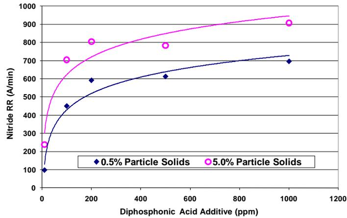
Figure 3. Nitride RR vs N1113 slurry additive level
