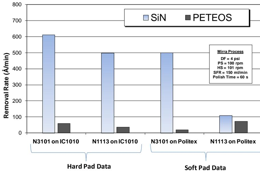
Figure 5. N1113 and N3101 polish data on hard and soft pads
