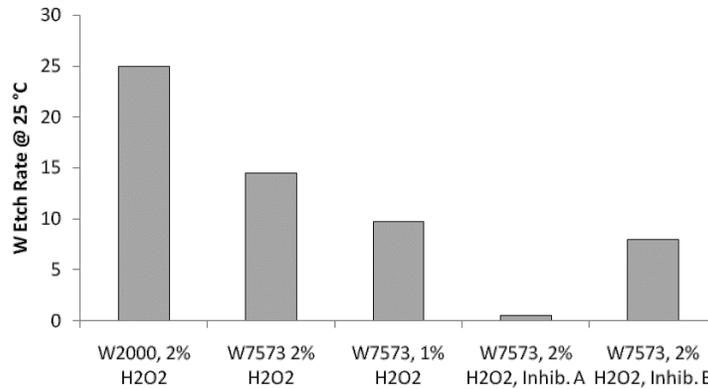
Figure 14. Tungsten etch rate vs. slurry for bulk polish slurries with varying oxidizer content and inhibitor type
