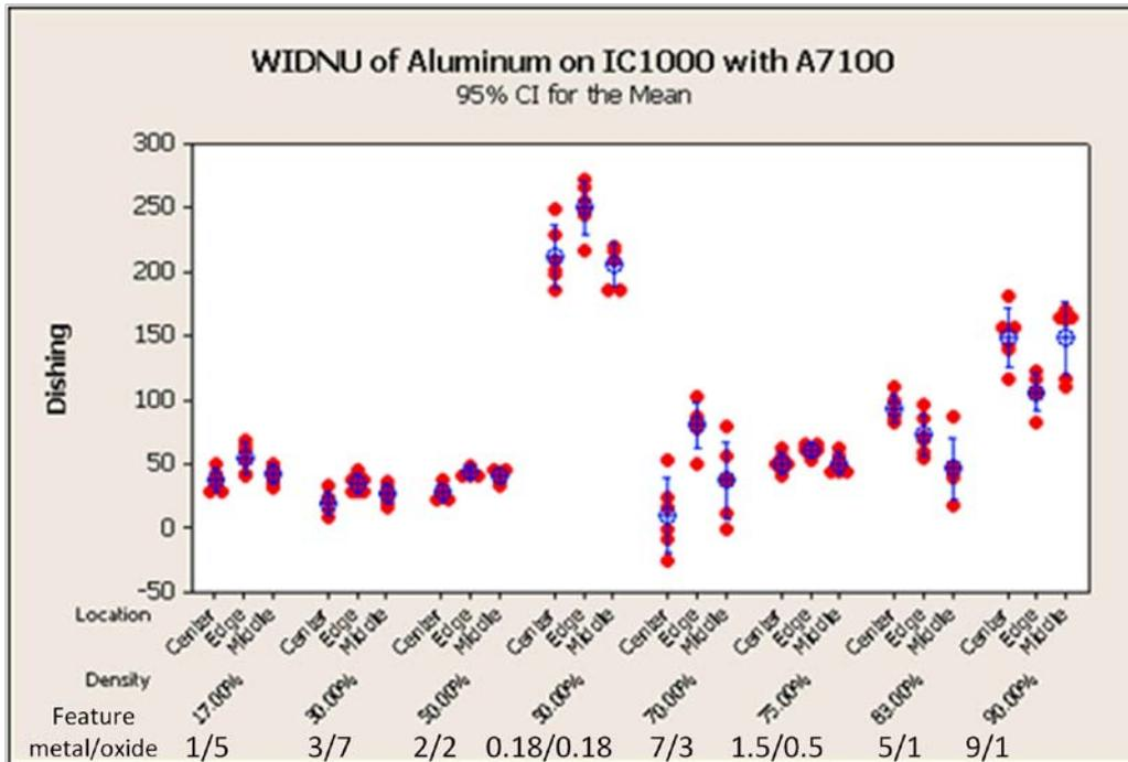
Figure 9. Comparison of feature dependent dishing between D100 and IC1000 pad with A7100 polishing slurry
