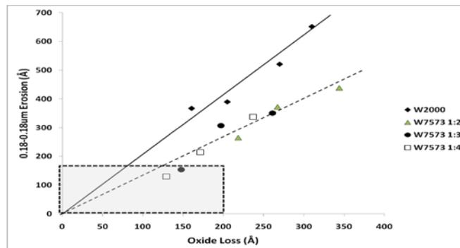
Figure 13. Oxide loss vs erosion for W7573 as function of dilution
